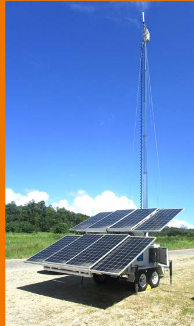
The OASIS Data Garden can be transported to any location in Solomon Islands to provide connectivity, electric power and a digital payment system for villages that are otherwise without access to electronic banking. ISIF Asia provided funding in 2021 under an inclusion grant to SATSOL, a local television and Internet provider.
